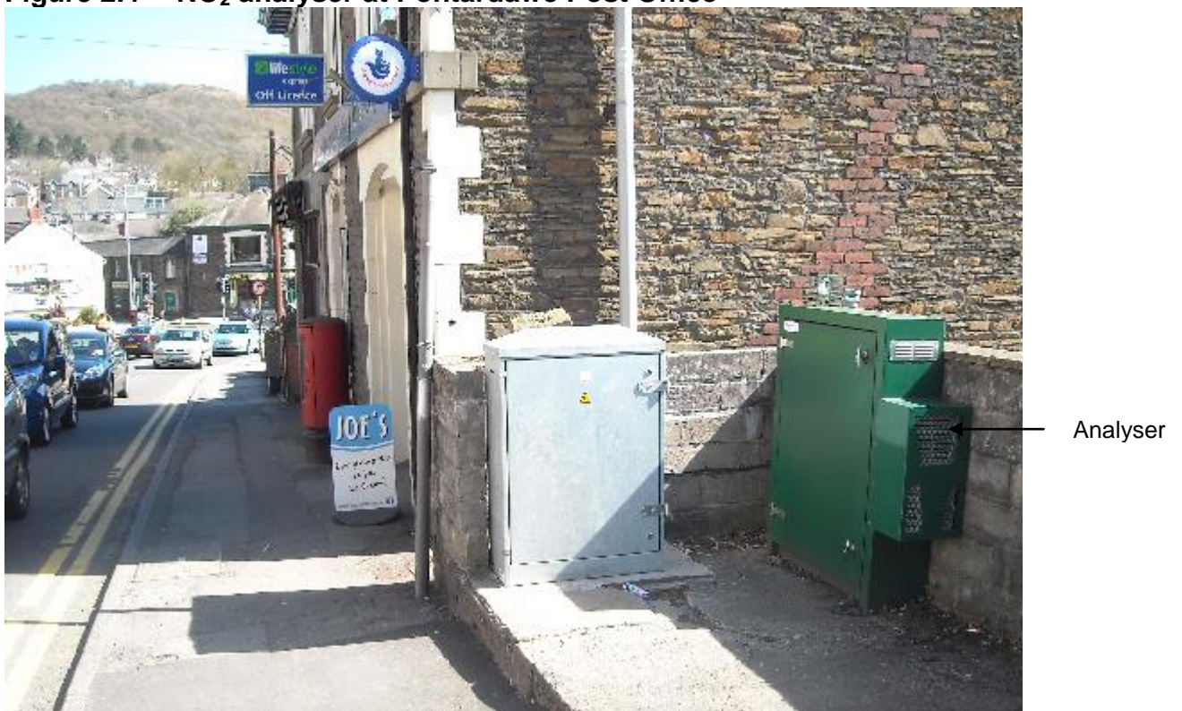
Figure 2.4 NO 2 analyser at Pontardawe Post Office
