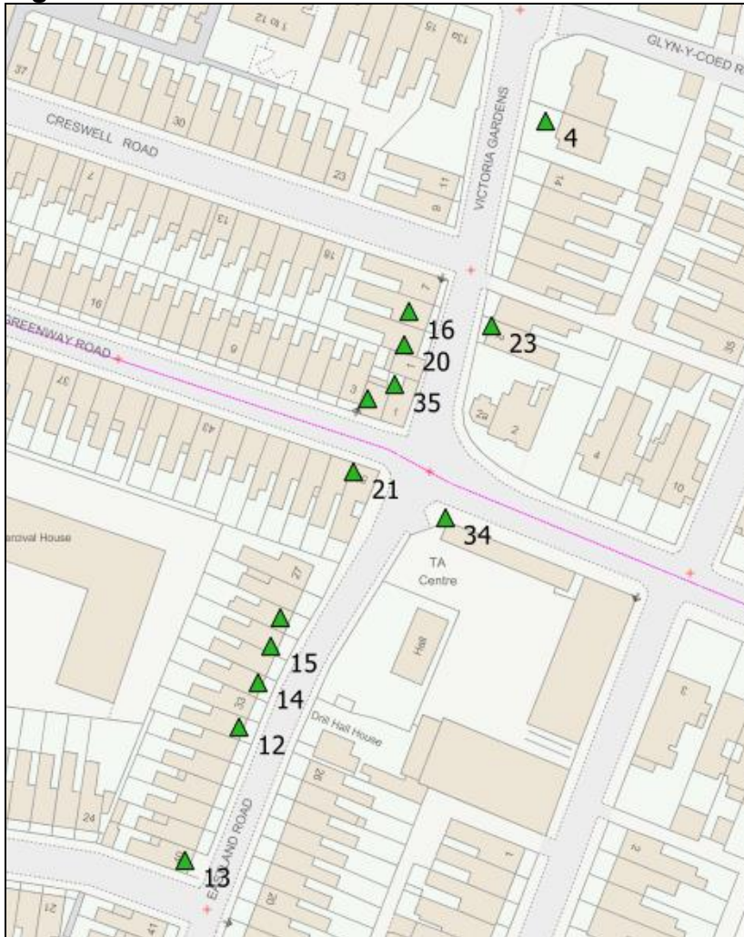
Figure 2.8 -Location of NO 2 diffusion tubes in Neath
